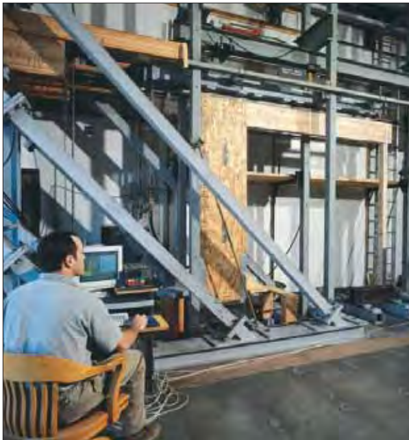
This test in the APA research center simulates seismic lateral loads over dozens of cycles to the same wall line. APA researchers can then determine the suitability of various bracing details for seismic performance, such as extending the header over the narrow end wall.
